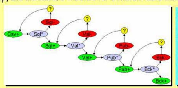
A state-machine representation of the loading process. Each step is a sequence of rather complex steps in itself. The yellow question marks represent a manual Undo step, which is performed as necessary.
